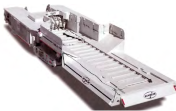
Figure 21-5. Example Three-Way Dump Feeder Breaker (from Joy 2010d)
